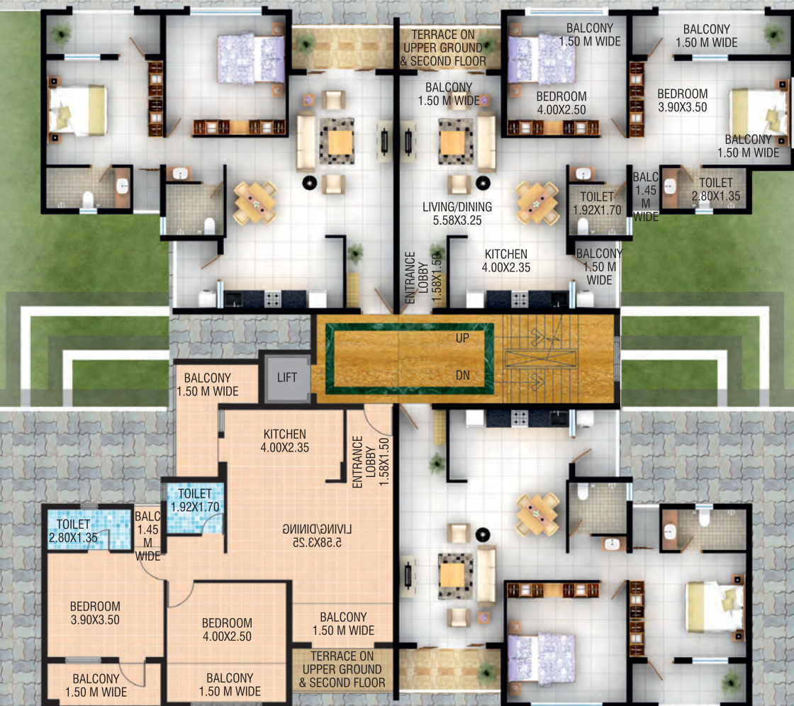
Typical Floor Plan for Block R
